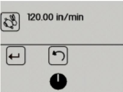
Figure 4: Setup screen for travel speed while welding.
